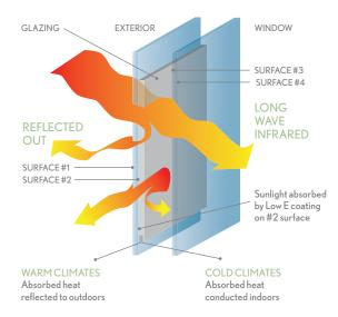
Low emissivety glass features a double metallic coating on the inside glass, which can reflect or absorb the sun's warmth to enhance either heating or cooling while reducing the effects of damaging UV rays.
